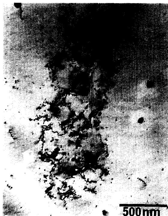
Fig. 2. An example of dislocation wall formation in pure copper irradiated with fission neutrons at 523 K [28] to a fluence level of 5 \times 10^{22} \text{ n/m}^2 ( 10^{-2} dpa, E > 1 MeV) [28].
